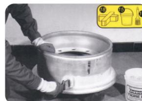
Put the rim on the wooden installation seat, then lubricate the rim.
