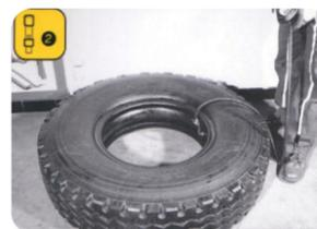
Remove valve core and in-flat for separating bead. Press the inner tube to squeeze air between the tire and inner tube, then screw on the valve mouth protector.
