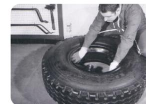
Put the hole of flap in the valve stem. Installed the belt between the inner tube and tire, and ensure the belt edge with no wrinkle or fold.
