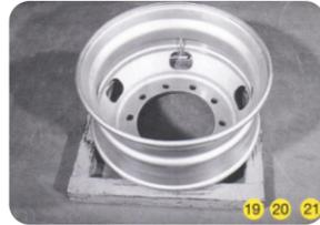
Using installation seat make it easier to install. Wheels must be down, the valve must be to the ground.
