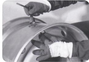
Install valve, clean metal parts and valve screw, keep them in a good state. Install valve to the correct place, use a wrench locking valve seat, then fix nut and fasten it.
