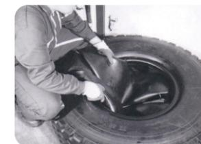
As shown, get the inner tube fold up and put into the tire.
