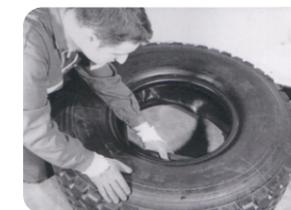
Open the inner tube and flattening in the tire.
