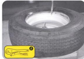
Install the other side of bead. Let tires slide to the other side. Make the flange be outside. Use holding forceps to clamp rim flange ring on the position of about ten centimeters from the valve.
