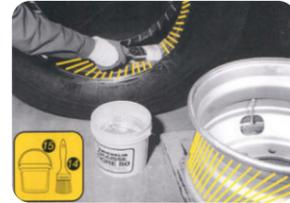
Lubricate the inside of the rim, bead and bead inside
