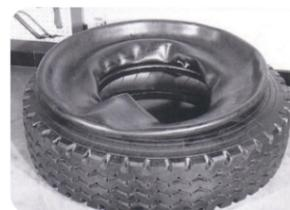
When it has inner tube ,put the tube on top of tire ,valve stem must be face up.
