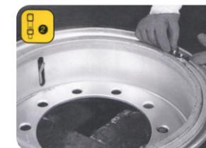
Make sure all components are installed correctly and cooperate with each other. If applicable, can be installed the safety clip, dismantling the valve protector, fitted with a valve core.
