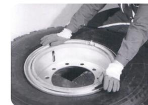
The following components installed, separate flange ring. Lock ring, the end with the valve into 180°.
