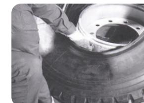
Incline the tire, insert the valve rod end into the valve groove, ensure that the valve is located in the valve groove center.
