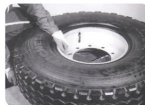
Push tires to rim, and make sure that valve is installed in the valve groove correctly.
