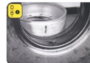
Screw on the valve cap, the tire loaded on the rim and put the valve in the groove.
