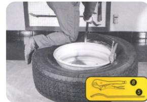
Press bead with your knee, and use the crowbar boost bead to the flange ring. Avoid pressure of bead, push the bead step by step. Unload holding forceps.
